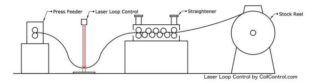
The above image depicts a typical customer setup utilizing a Laser Loop Control to modulate the speed of the straightener by measuring the loop between the straightener and press feed.
